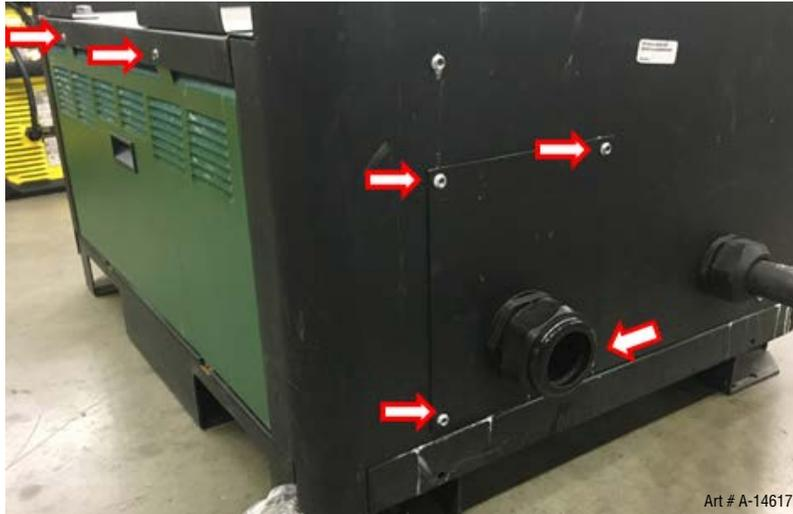
2. Carefully cut back the outer sheath on the primary input power cable to expose the individual wires. Cut back the insulation on the individual wires. Route the power cable through the strain relief and attach the 3 phases to L1, L2, L3 and the green/yellow earth ground wire to ground terminal accessible through the side panel.
