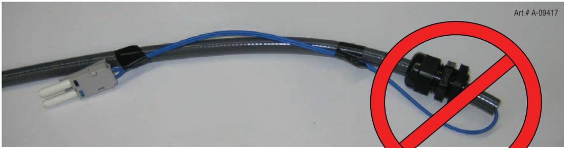
2. Don't hook onto the fiber to pull on the cable.
