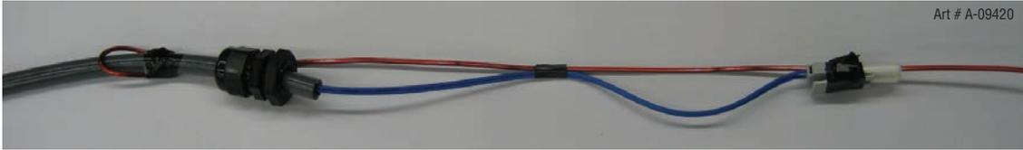
Correct installation in CCM or Gas Control leaves a loop of fiber so there is no stress on the fiber where it exits the connector or the hose.
