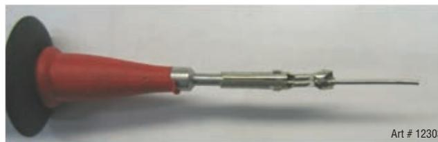
Insulate all but the end of the wire and slide these onto your meter probe. If your meter has alligator clip adaptors you could hold the wire in these as well, be sure they don't short together.
