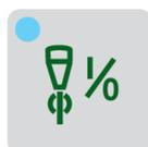
Pressing the TORCH ON / OFF button when manual mode is activated, will either manually start or turn off the cutting process.
