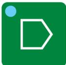
Sends the cutting program from the “next job preview” screen to the “current job” screen to be executed, and starts the cutting cycle sequence. The START- button illuminates and is on during the entire execution of the program. No programs can be transferred to the current job screen if the START button is on.
