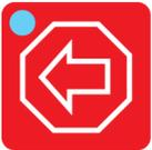
Press and release the STOP BACKUP button once during the cutting process to stop the cutting sequence and halt machine motion. Press and release the STOP BACKUP button again to move the machine in reverse, or backup on path. Pressing STOP BACKUP button again will stop motion.
