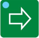
The MOVE AHEAD button is illuminated whenever a program is running. Pressing the Torch On/Off button will stop the machine and the Move Ahead button will turn off. At this point, pressing the MOVE AHEAD button will cause the machine to move forward on programmed path without cutting. Pressing the MOVE AHEAD button again will stop machine motion.
