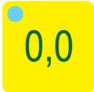
Resets the X & Y counters to ZERO after locating a new starting point on the table using the jog function keys.
