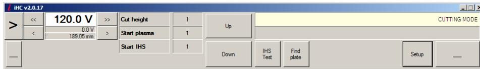
The large right pointing arrow can be used to make the iHC main bar smaller. This allow operator to see position and other information about the machine.
